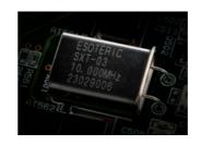
The raw crystal material is slowly grown over a long period of time and then SC-cut (Stress Compensated Cut) with excellent temperature characteristics. We also scrutinize the manufacturing process down to the smallest detail, carefully selecting and using crystals whose center frequency fluctuations are strictly within specifications.
